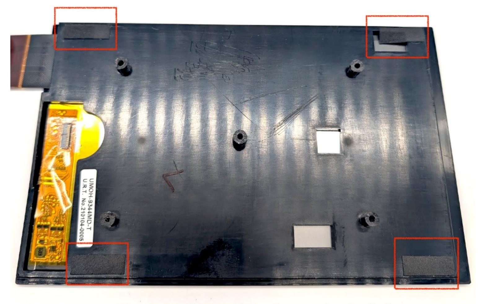
Remove Foam Tabs for easier install.
